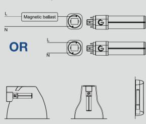
**DIRect or BYPass Installations - 2 Pins Mode**
