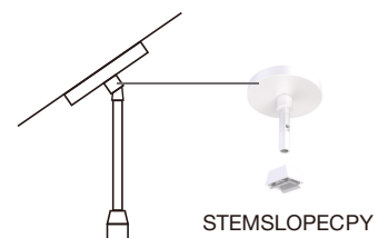
Pendant Mount Installation - Slope Ceiling (front side view)
