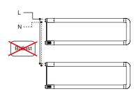
Not polarity sensitive, lamps can be wired at either end.
