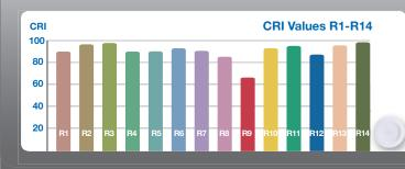
The CRI<sup>SP</sup> SERIES DOWNLIGHT 12W lamp features a typical CRI 90, R9 64 and R13 95, providing crisp and vibrant colors across the whole spectrum. Its exceptional R9-R14 values (R9 & R13) provide redder reds, natural looking skin tones and whiter whites. In addition, this lamp's color temperatures fall within a 4-step Macadam ellipse to ensure minimal color deviation across lamps.
