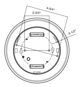
Suitable for installation in junction box with mounting holes spacing dimensions of 2-3/4", 3-1/2" and 4-3/4".
