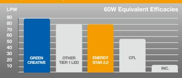
60W replacement industry average and exceeds new ENERGY STAR 2.0 requirements. This energy-saving performance makes this lamp a smart retrofit choice for incandescent and CFL bulbs.
