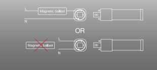
When used with a magnetic ballast, the PL H can function as a plug & play lamp and operate with the existing ballast. If the ballast is not compatible, it can be bypassed and the lamp can run directly off line voltage.
