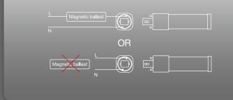
When used with a magnetic ballast, the PL H can function as a plug & play lamp and operate with the existing ballast. If the ballast is not compatible, it can be bypassed and the lamp can run directly off line voltage.
