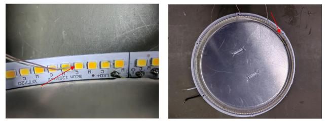
Temperature measurement point of LED light source (TMP<sub>LED#2</sub>)
