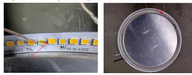
Temperature measurement point of driver (TMP<sub>c</sub>)
