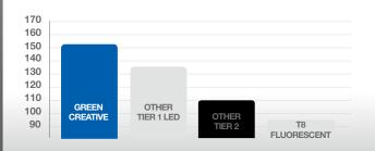
At 152 LPW, GREEN CREATIVE's ultra-high efficacy T8 BYP tube is 16% more efficient than the Tier 1 LED T8 industry average. This energy-saving, high-performance T8 is a smart retrofit choice that provides a faster ROI than traditional T8 LED tubes.
