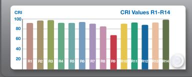
The CRISP SERIES DOWNLIGHT 10W lamp features a typical CRI the whole spectrum. Its exceptional R9-R14 values (R9 & R13) provide redder reds, natural looking skin tones and whiter whites. In addition, this lamp's color temperatures fall within a 4-step Macadam ellipse to ensure minimal color deviation across
